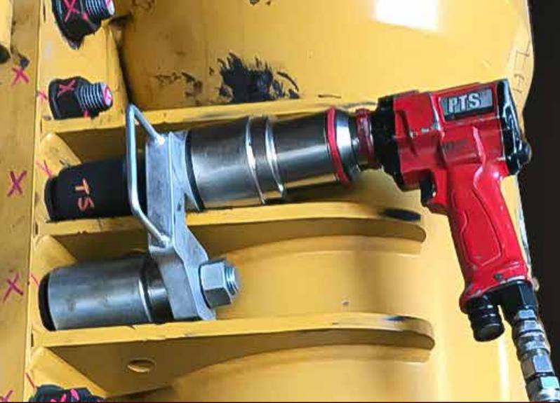
*The SPL541 reaction arm and PTS tool offer a stable and safe reaction force transfer between the nut being tightened and the adjacent nut.*
