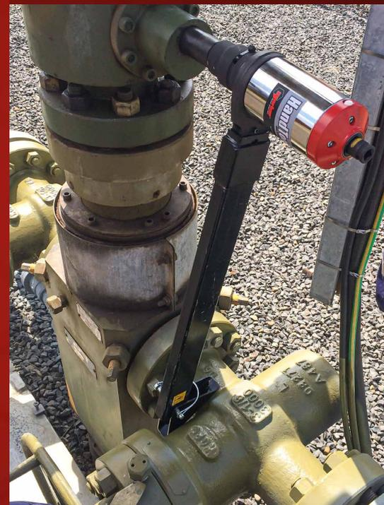
*Image: The SPL404 reaction arm extended to react upon the body of a wellhead. It can be extended to use a nearby surface as a reaction surface.*
